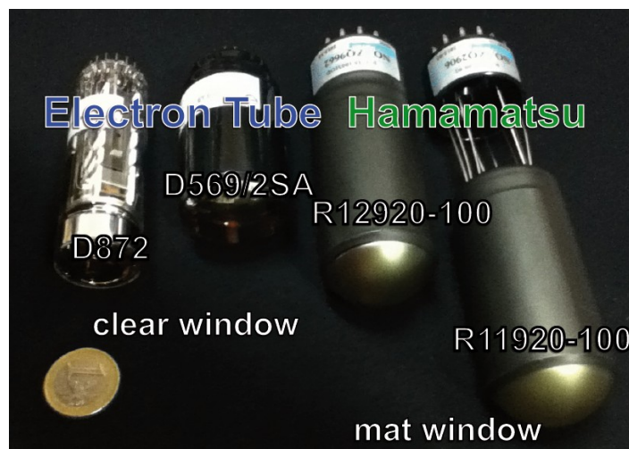
Figure 1. Photo of candidate PMTs for CTA. Left: prototype test-bench PMT D872 from ETE; 2 nd from left: 8-dynode PMT D569/2SA from ETE, 3 rd from left: 7-dynode (final) PMT R12920-100 from Hamamatsu; 4 th from left: 8-dynode PMT R11920-100 from Hamamatsu. Note that the PMTs from Hamamatsu have a mat input window.
