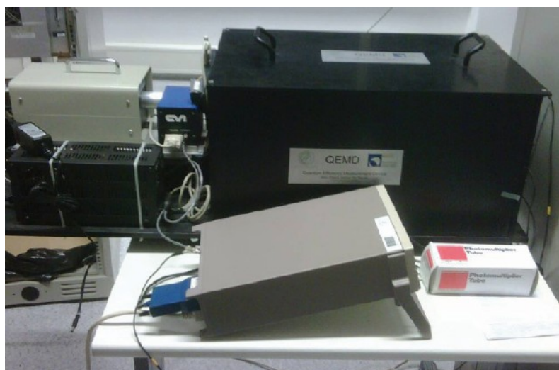
Figure 2. QE measuring custom-designed device in MPI. On left top one can see the light source (grey box) accommodating a deuterium and a halogen lamps, the small blue box is a modified spectrometer. Light from it enters into the sensor test dark box via a filter wheel. In front is shown a Keithley Picoammeter (grey) of type 6485.
