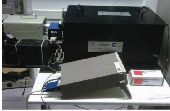
Figure 2: Custom designed QE measurement device at MPI. The grey box at the top left contains the light source (deuterium and halogen lamps). The small blue box is a modified spectrometer. Light enters into the dark box containing the sensors (right) via a filter wheel. In front a Keithley Picoammeter model 6485 is shown.
