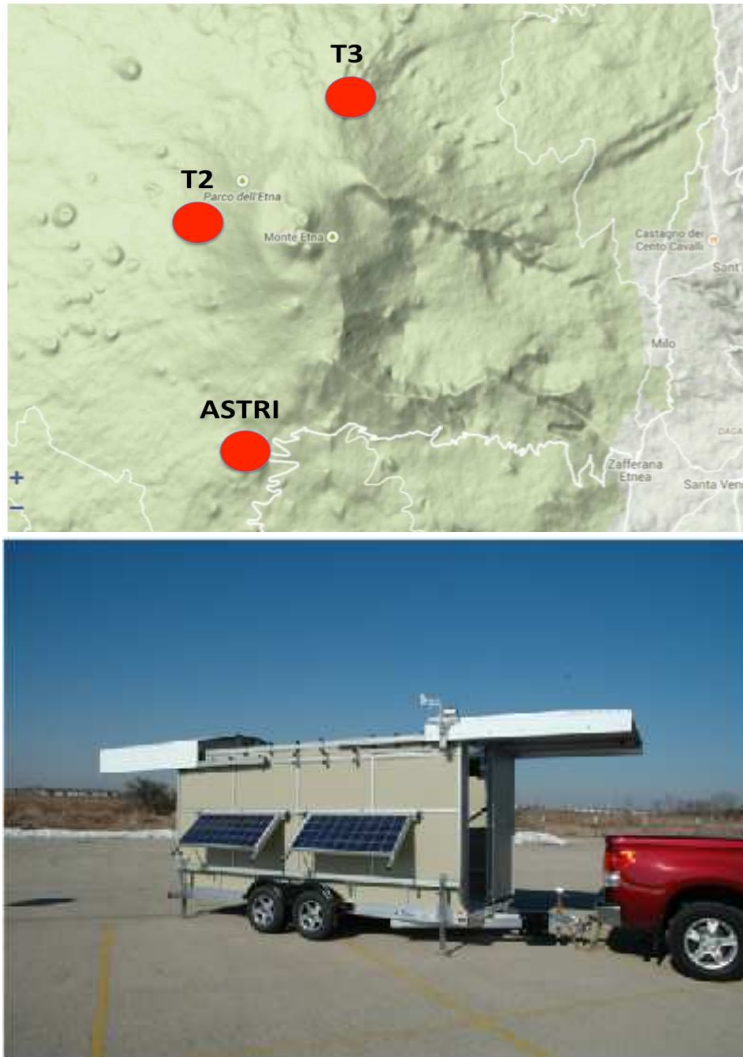
Figure 11: Top : A possible Cherenkov telescopes configuration for the Mt. Etna tomography. Bottom : An example of trailer that could be used for hosting the telescope and moving it in different Etna observing sites.
